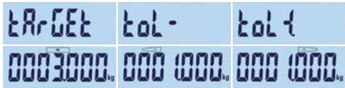
Figure 5-2: Target and Tolerance Displays: Target (left), Low (center) High (right)
